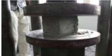
Fig. 1. Compressive Strength Test
