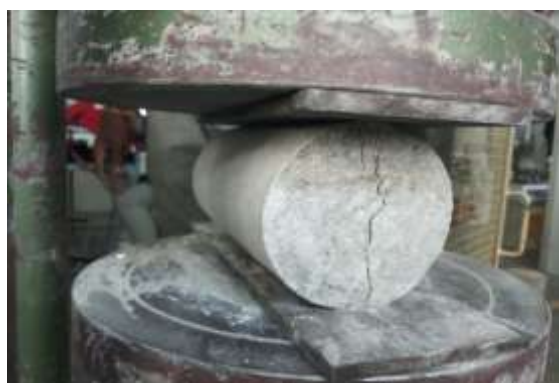
Fig. 5. Split Tensile Test
