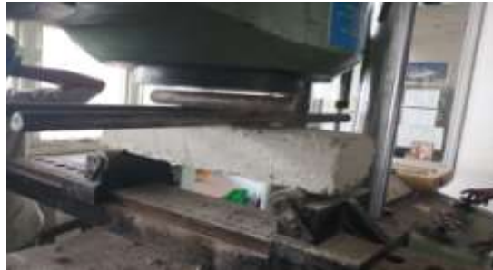
Fig. 7. Flexural Strength Test
